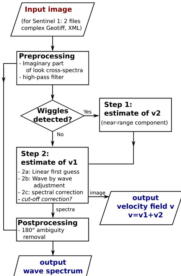
Figure 2: Different steps in the image processing that are detailed in the following subsection. The possible cut-off correction appears in *italics* because it has not been implemented yet and its feasibility is discussed in section 3. Without this cut-off correction the wave amplitudes of the  $v_1$  component can be underestimated near the ice edge.
