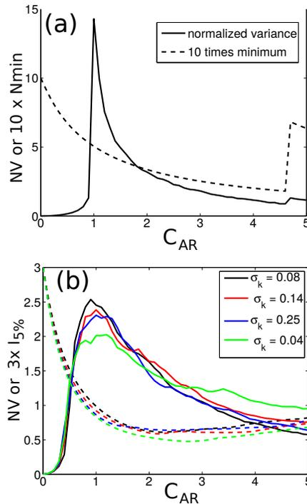
Figure 4: (a) Variation of the normalized image variance and normalized minimum intensity in the case of a monochromatic wave of amplitude  $a$  traveling along the azimuth direction, as a function of the SAR mapping nonlinearity parameter. (b) Similar variation but for a Gaussian wavenumber spectrum  $E(k) \propto \exp(-((k - k_0)/\sigma_k)^2/2)$ , with  $C_{AR}$  defined from the r.m.s. wave amplitude.  $I_{5\%}$  is the mean intensity of the 5% less intense pixels, shown with dashed lines.
