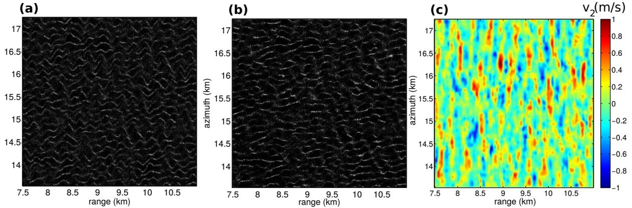
Figure 3: Illustration of the first step: the original image in (a) is transformed in (b) by an inverse SAR transformation given by eq. (3) using the velocity field  $v = v_2$  shown in (c). The straightening algorithm works best for sharp and bright features, e.g. around  $x = 7.7$  km,  $y = 14.2$  km. The linear gray-scale for the image intensity goes from 0.5 to 8.
