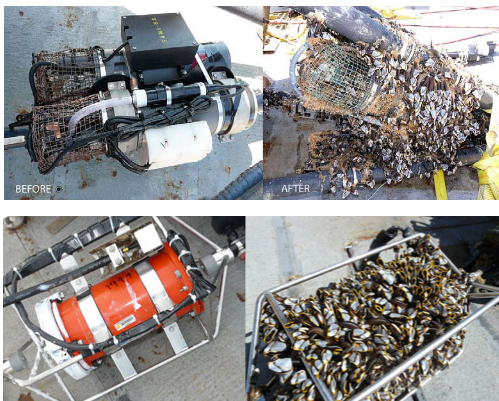
Figure 3.3: Some examples of biodeterioration effect on sensors ( www.stccmop.org/blog/schillij/biofouling ).
