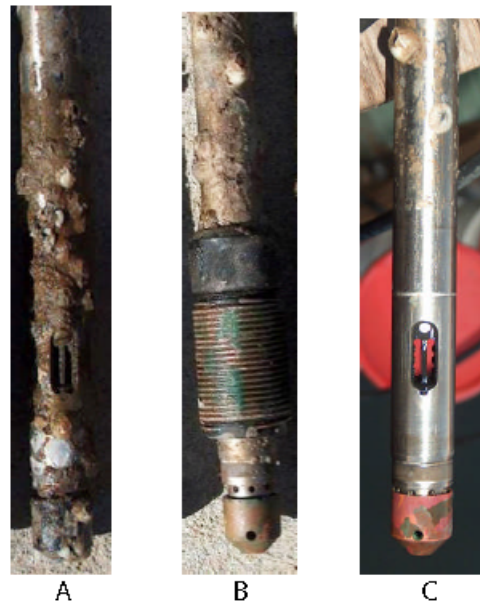
Figure 4.13: The Aqua TROLL 200 control (A) and the Aqua TROLL 200 with TROLL Shield guard and nose cone (B). In C the nose cone is in place and guard removed to show how effectively it protects the conductivity cell from biofouling. The conductivity cell was not cleaned.
