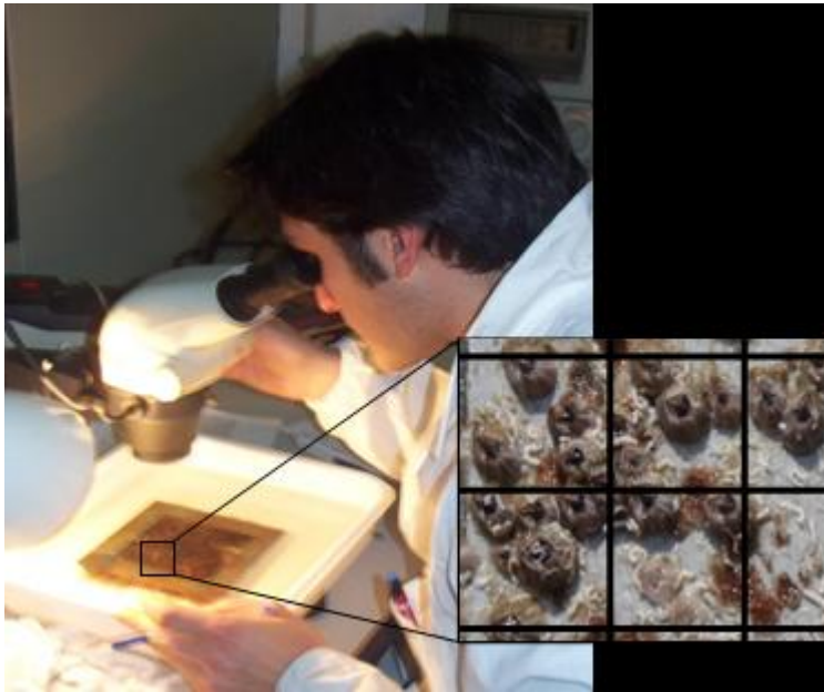
Figure A.3.2: Estimation of fouling by standard microscopy techniques and Dethier method.
