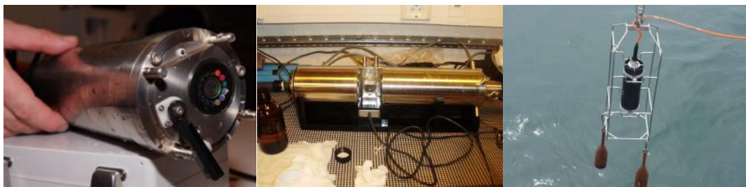
Figure. 3.2.4. Commercial spectral fluorometers: Multiexciter (left), FluoroProbe in lab measurement mode using Workstation (middle) and FluoroProbe in profiling mode (right).
