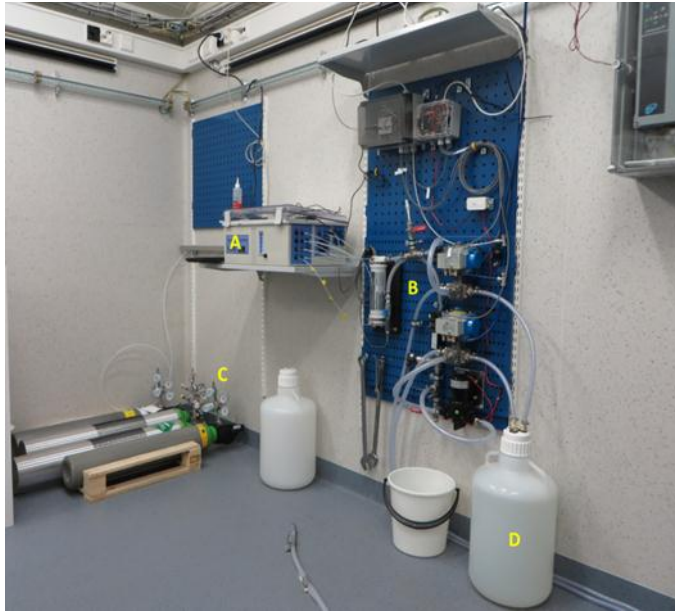
Figure 3.3.3. SuperCO 2 measuring system at Utö Atmospheric and Marine research station. (A) instrument, (B) equilibrators and valves, (C) calibration gases and (D) container for cleaning agent.
