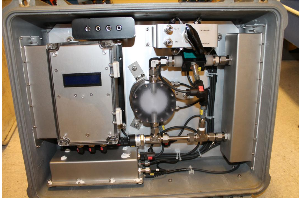
Figure 3.3.2. An example of a Franatech pCO 2 sensor system. The leftmost part contains the electronics, datalogger and display. The circular object in the middle is the equilibration chamber. And the detector lies along the bottom of the case. Water inlet and outlet on the right side of the unit with water pressure and water detector mounted. On the top the gas interface for calibration.
