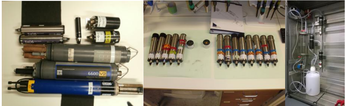
Figure. 3.2.2. Examples of LED fluorometers from different manufacturers (left), during calibration exercise (middle) and installed on flow through system (right).
