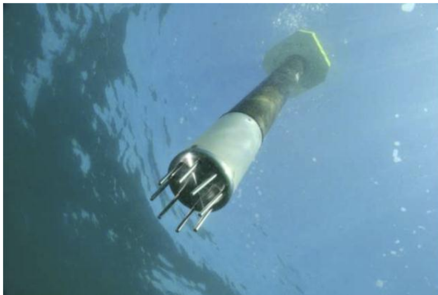
Figure 3.4.1 Arvor-C during the descent. On the bottom end, its claws prevent drifting when grounded on the seafloor (Photo credits : Olivier Dugomay – Xavier Caisey (Ifremer))
