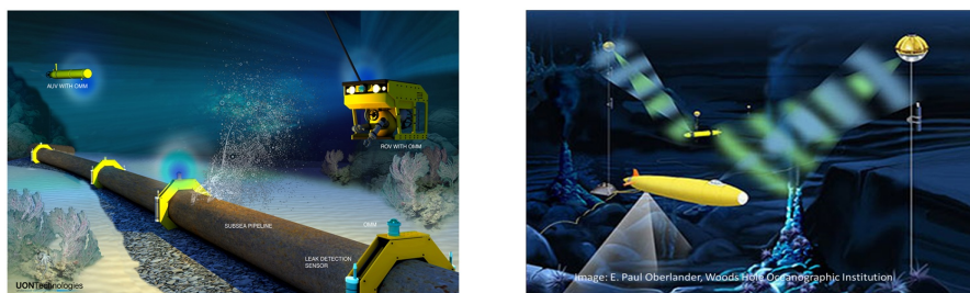
(a) Underwater oil and gas pipelines monitoring with UWOC networks [20].
