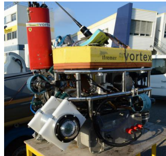
Figure B.4: Transmitter Ifremer's Optical modem integrated on Vortex.
