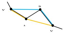
Speeds on the segments X-A-Y (orange trajectory) and X-B-Y (blue trajectory) are computed. If speed<sub>X-A-Y</sub> is greater than speed<sub>X-B-Y</sub>, the position A is defined as 'abnormal' by the speed test otherwise B is defined as 'abnormal' by the speed test.
