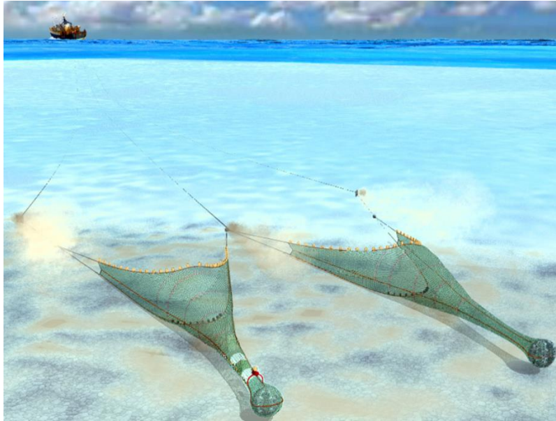
Figure 4.2.2.5 Twin trawl gear where the fishing performance of a test gear is compared with that of a standard or control gear
