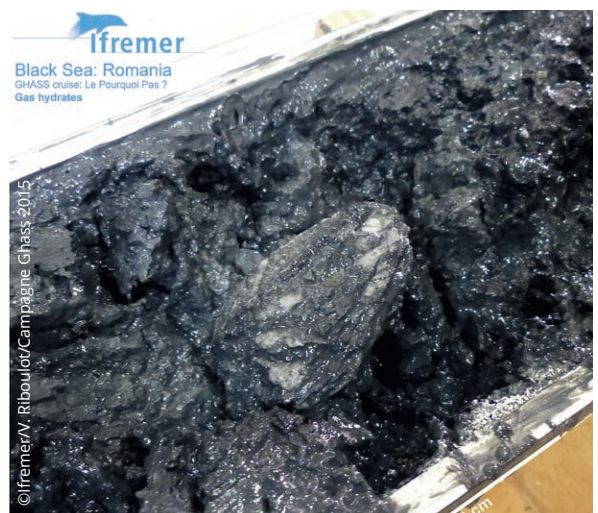
A core sample taken in the Romanian sector of the Black Sea during the Ghass mission, showing the presence of gas hydrates for the first time (at centre)
