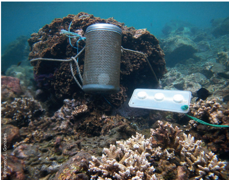
Pocis (metal cage) and DGT (white plate) passive samplers submerged in the lagoon environment
