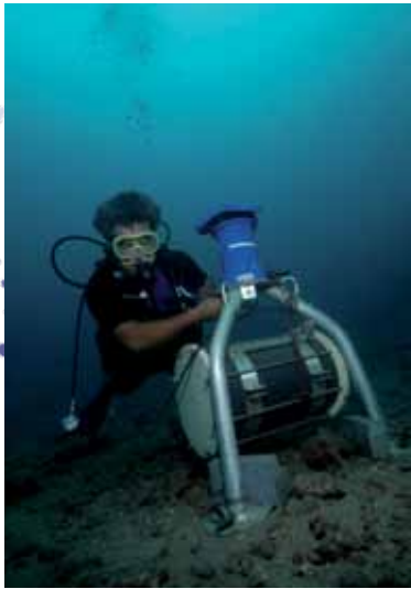
Current measurements with an ADCP profiler (Tahiti lagoon)
