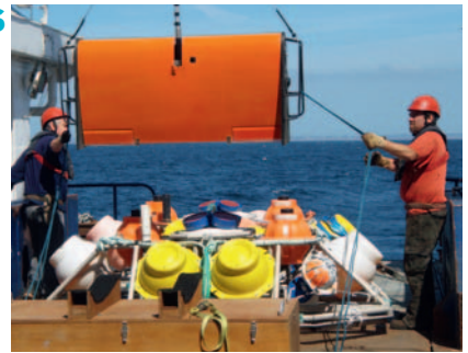
Various steps to launch Scanfish deployed during the Aspex cruise
