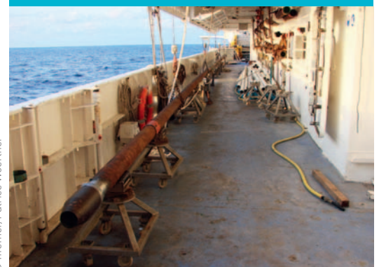
33-metre long core sample taken at depth of 4,963 m during Reprezai-1 cruise
