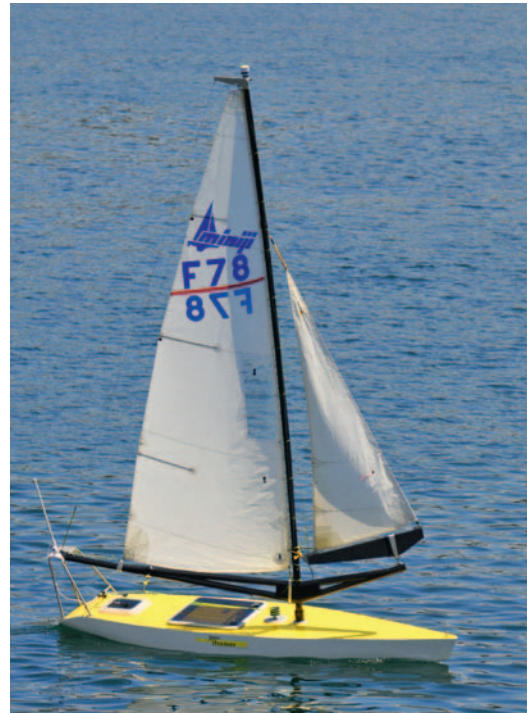
Sailing robot Vaimos - Autonomous sailing boat with embedded instrumentation - using wind power and solar energy for measurement and observation missions at sea
