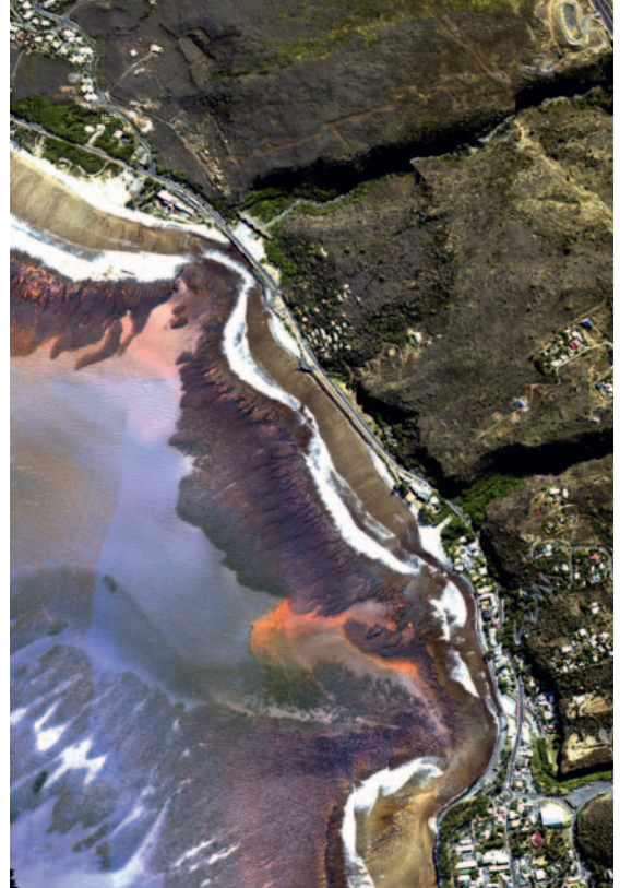
Hyperspectral image (corrected for water column effects) highlighting the characteristics of outer reef slopes to depths reaching 30 metres in the bay of Saint-Leu/Reunion Island
