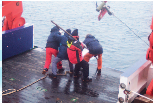
Recovering one of the moorings equipped with current meters off Greenland
