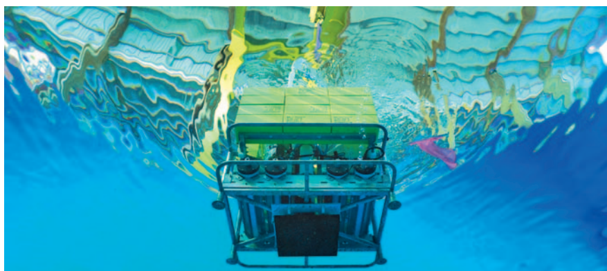
The autonomous "BOB" bubble observatory module lander in the Brittany centre's test tank
