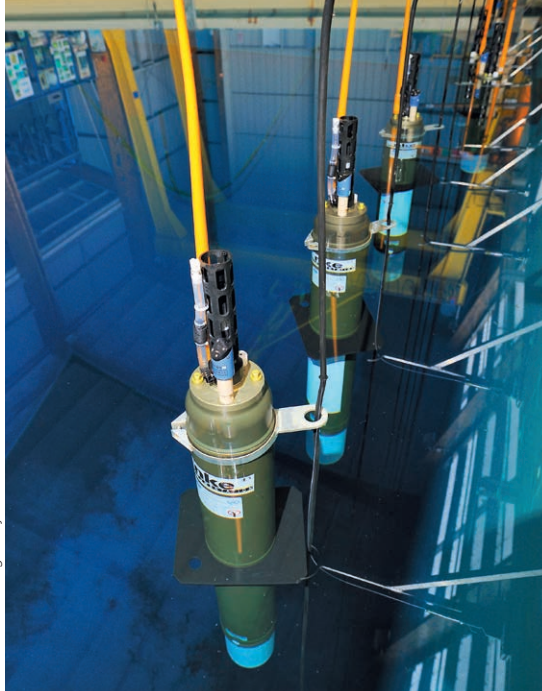
◀ Testing profiling floats with an oxygen probe in the test tank at the Ifremer centre in Brest
