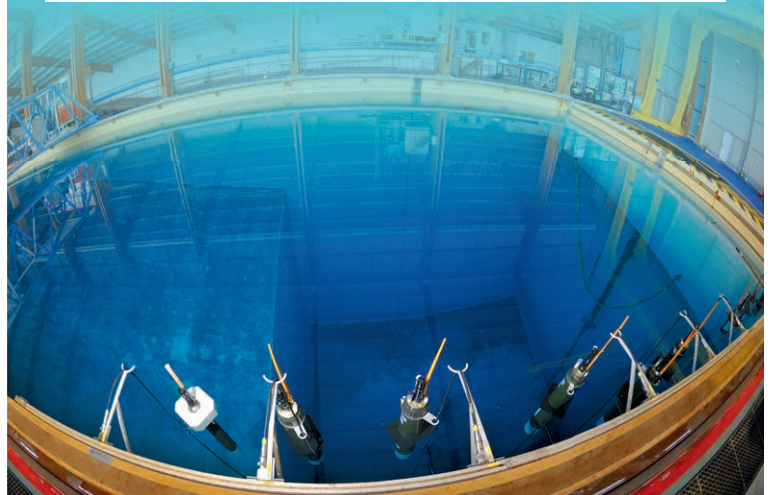
▲ Testing Provor (profiling) floats Provor (with oxygen probe) at the test tank in the Ifremer centre in Brest
