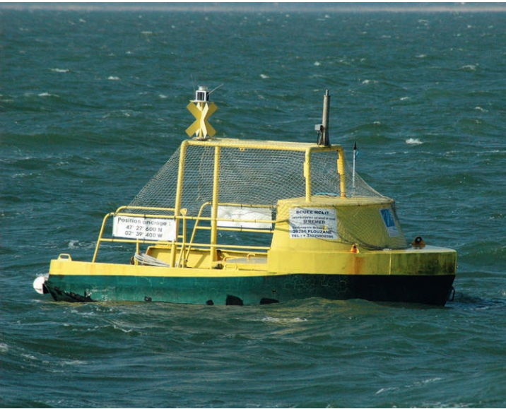
Sea deployment of the Molit buoy, a measurement station for continuous monitoring of marine water quality parameters
