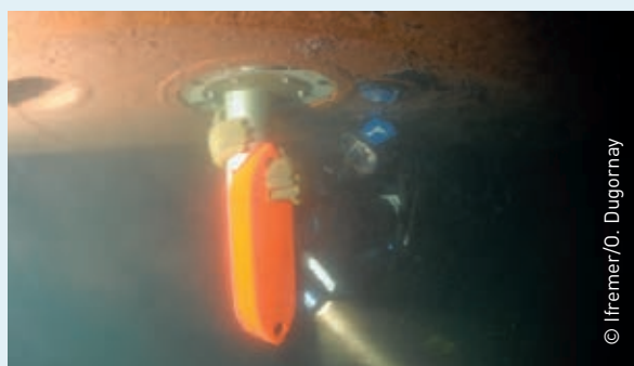
→ Inspection of acoustic bases and hull of RV Thalassa by divers
