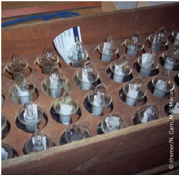
→ Samples to measure dissolved oxygen to study variability of currents and water bodies
