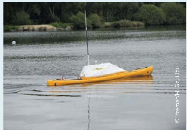
→ Mobesens: mobile autonomous system to measure water quality
