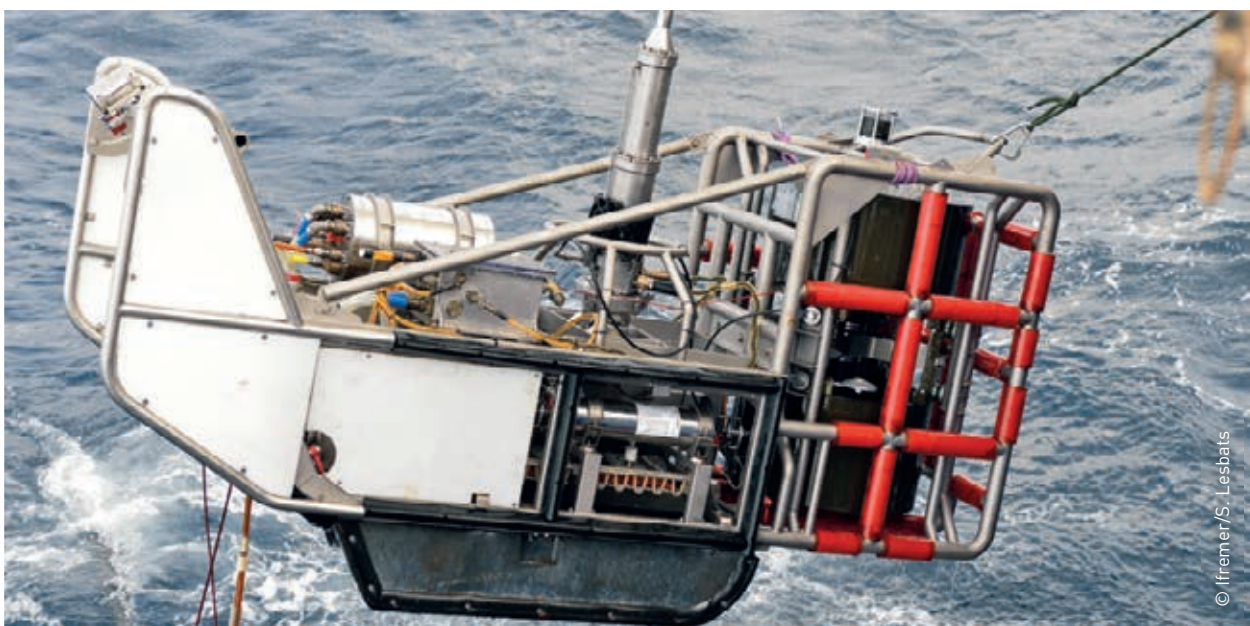
→ Retrieval of Sysif near-bottom seismic module
