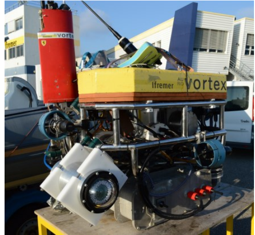
Fig.3. Ifremer's transmitter prototype integrated on Vortex
