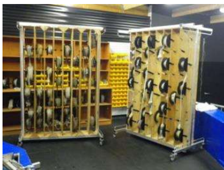
Figure 2 : trawl models fitted for the Lorient flume tank
