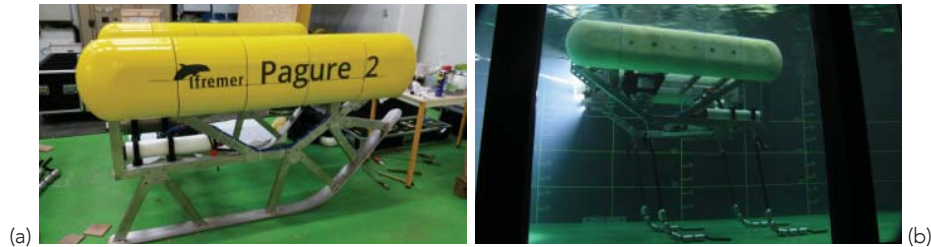
Fig. 1. View of the Pagure-2 on 'sledge' mode with its skates (a) and on 'flying' mode with flexible weights (b). (© Ifremer, J.V. Facq).
