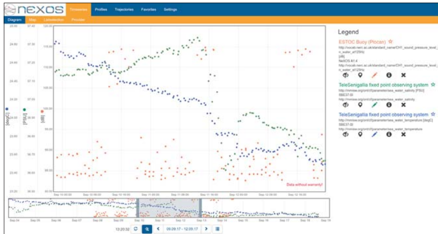
Fig. 2. Example of a data presentation from the SWE user front end viewer developed by 52oN. In this case, data from the ESTOC buoy by Plocan: sea temperature (blue dots), salinity (green dots) and sound level (orange dots).
