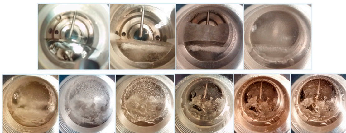
Figure 4. Top panel: Visual observation of the evolution of the different phases during gas hydrate crystallization (from left to right: directly after water injection; after stirrer has been set to 400 rpm; 1 min after the gas hydrate formation incipient; 48 min after the gas hydrate formation incipient). Bottom panel: Visual state of the system during the gas exchange process (from left to right: t = 0 h; t = 1.47 h; t = 18.90 h; t = 89.73 h; t = 118.90 h; t = 145.73 h).
