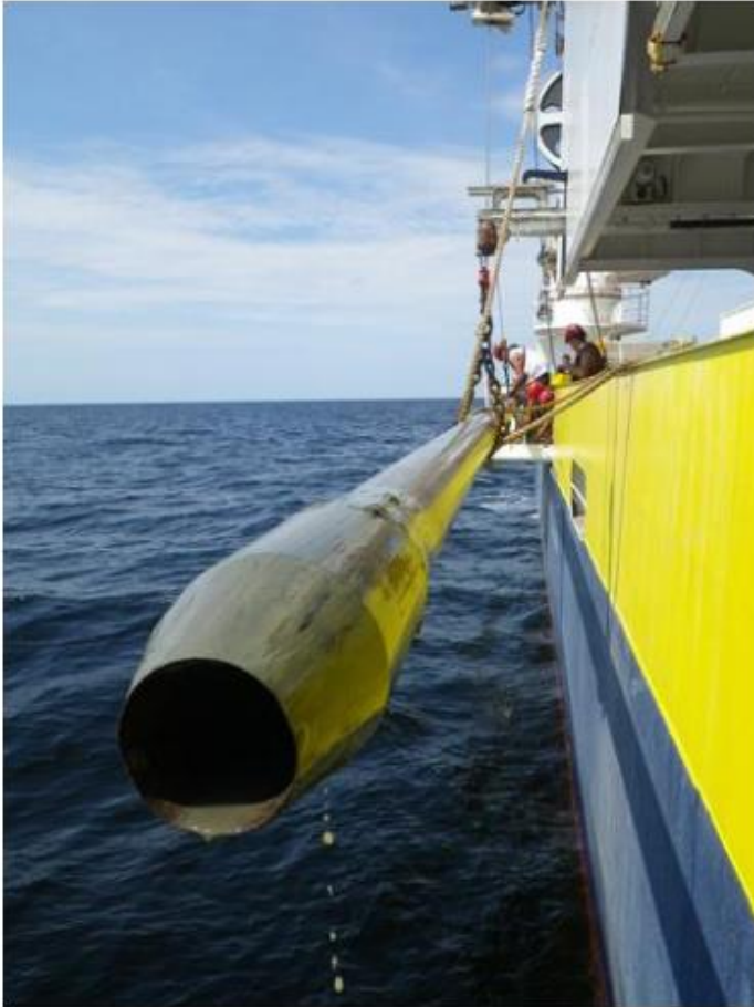
Kullenberg Calypso Corer (minimal sediment perturbation)
