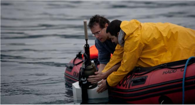
© Antoine Poteau, Observatoire Océanologique de Villefranche (CNRS/UPMC) Deployments of a bio-Argo Provor in Ligurian sea
