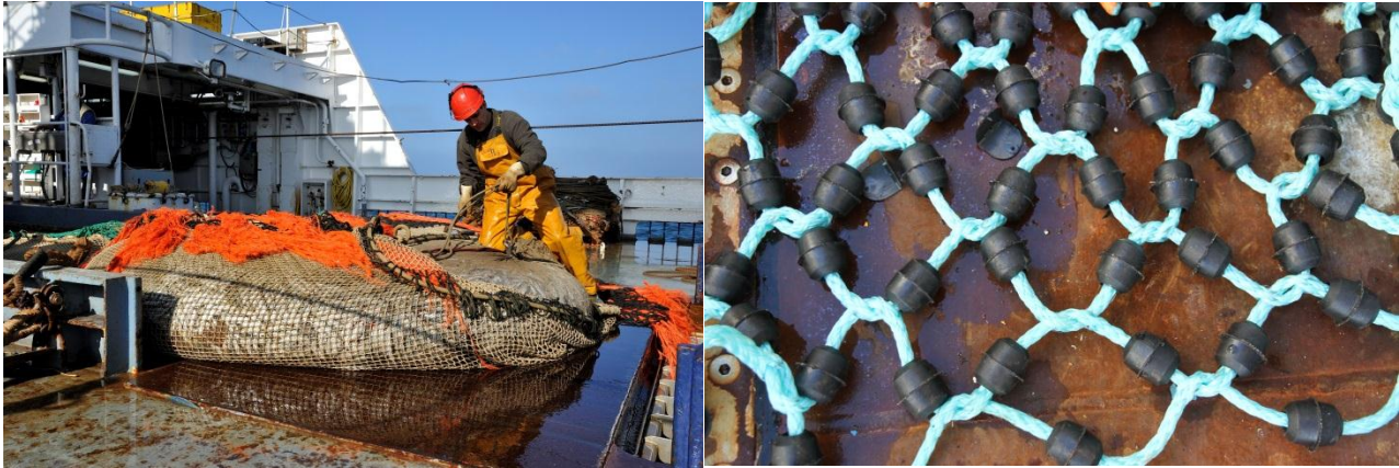
Figure 2. Onboard RV Thalassa the codend protective (orange) layer made of polyethylene twine (left) has been replaced by a rubber mat (right) to reduce plastic fibre pollution.
