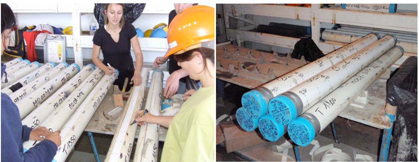
Figure 21: metric tape is stuck on the sections and the caps and fixed with duck tape (photos: N. Dubois and R. Biville).
