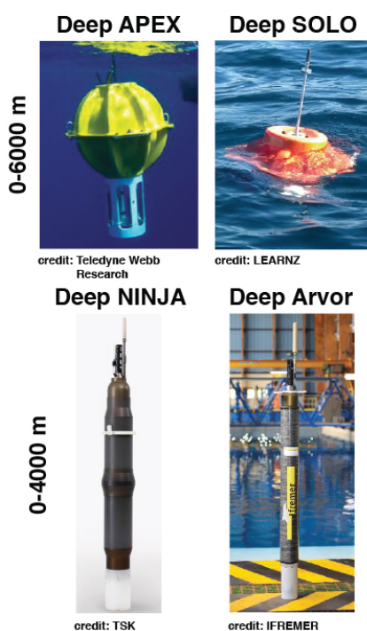
Figure 3: The four Deep Argo float models: the Deep APEX floats, developed by the University of Washington and Teledyne/Webb; the Deep SOLO floats, developed by Scripps Institution of Oceanography; the Deep NINJA floats, developed by Japan Agency for Marine-Earth Science and Technology (JAMSTEC) and Tsurumi-Seiki Co. (TSK); and the Deep Arvor floats, developed by Institut Français de Recherche pour l'Exploitation de la Mer (IFREMER), Centre National de la Recherche Scientifique (CNRS), and nke Instrumentation.
