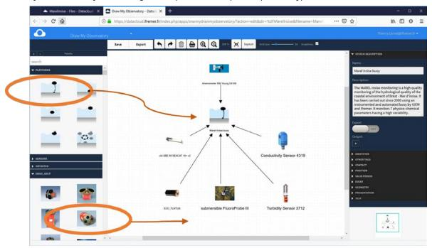
To connect a sensor to the platform, click on the sensor icon, on the right arrow, hold the click and go to the platform.
