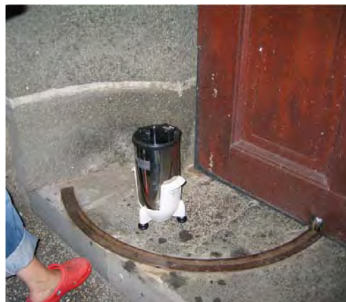
Picture 3b : Gravity measurements at "Port des Galets - Eglise" (reference point) using SODIN portable gravimeter.
