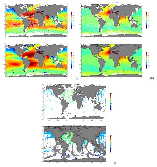
Figure 17 SDC\_GLO\_CLIM\_V1\_1 August Salinity Climatology in PSU: a) at surface; b) at 950 m, and c) at 3750.
