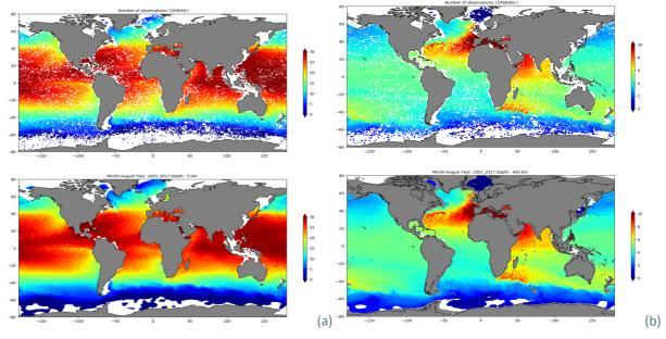
Figure 15 SDC\_GLO\_CLIM\_V1\_2 August Temperature field in Degree C: a) at surface; b) at 950 m.
