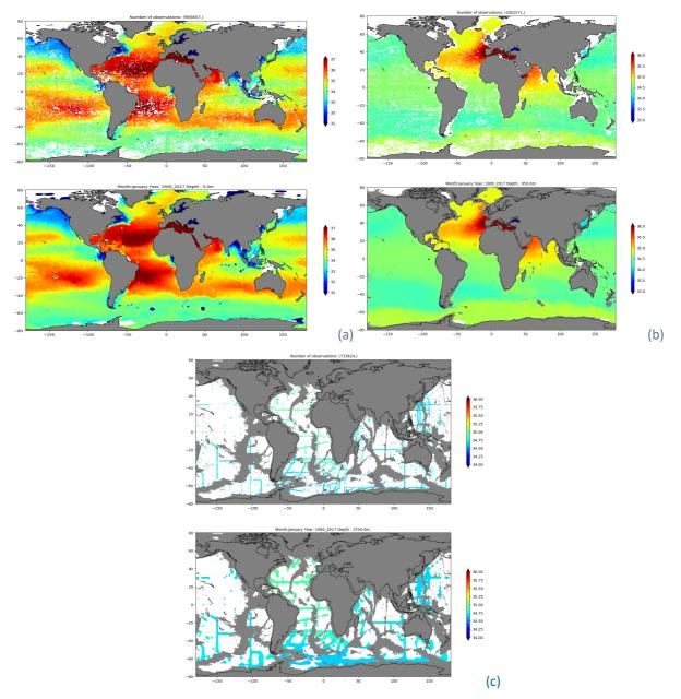
Figure 16 SDC\_GLO\_CLIM\_V1\_1 January Salinity Climatology in PSU: a) at surface; b) at 950 m, and c) at 3750.
