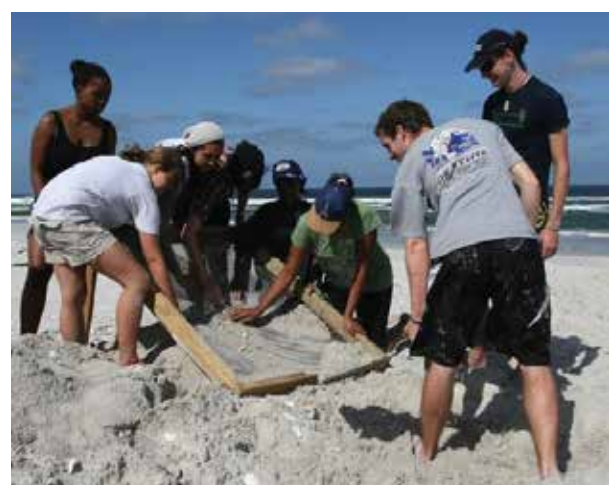
Figure 4.12. Sampling buried macro-litter on a sandy beach, using a team of students to sieve the top 15 cm of sand from a 1-m wide transect running up the beach profile (see Figure 4.3). (©Peter Ryan).
