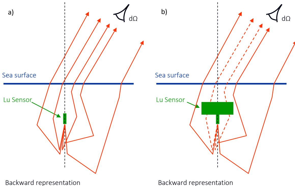
**Figure e : description of the shading estimation method using two Backward Monte Carlo Simulation. a)** First simulation with a transparent sensor. **b)** Second simulation with a real sensor which obstructs photons trajectories.
