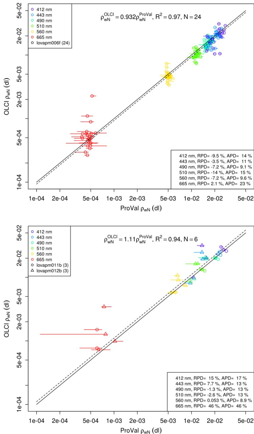
Figure d : normalized reflectance  $\rho_{wN}$  from OLCI and ProVals for top: Mediterranean (*lovapm006f*) and bottom: Southern Ocean floats (*lovapm011b* and *lovapm012b*). Error bars on the ProVal data are given by the minimum and maximum of the four normalized reflectance values. Solid line represents the 1:1
