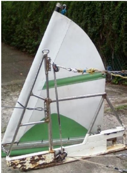
Figure 8.16.2. The bat wing otter board. This otter board is designed to be operated at an angle of attack of around 20 degrees, during trawl deployment and while on the seabed. In this way lift to drag ratio is optimised without compromising stability.
