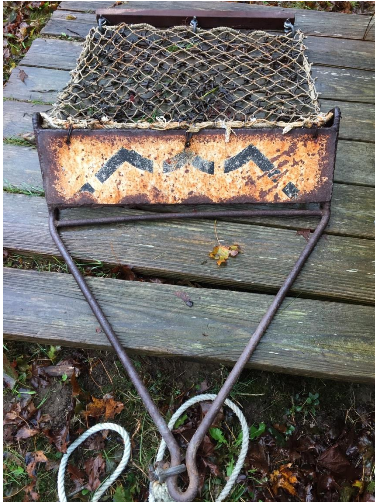
Figure 8.15.11: A typical bay scallop dredge. Width is approx. 0.8 m
