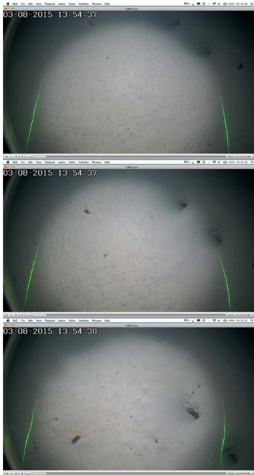
Figure 5.12. FU3-4: Still image of video footage showing the misinterpretation where the stripe laser appears to bend around burrows. In this case the burrow on the far right hand side is not counted.
