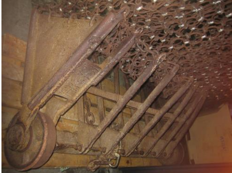
Figure 3. Roller dredge used in the Chlamys islandica fisheries in Breiðafjörður.
