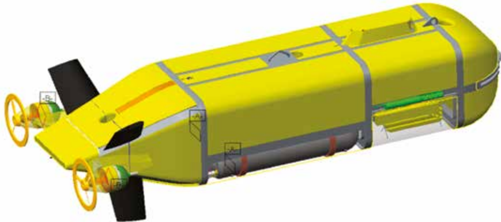
6000m AUV for wide scale survey and local inspection developed at Ifremer
