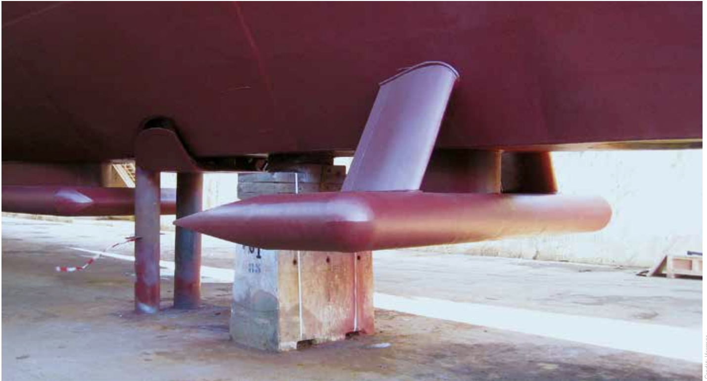
Gondola fitted to the hull of RV L'Atalante
