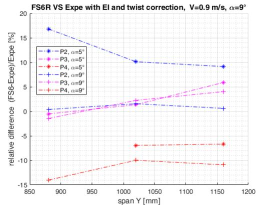
Figure 17: FS6R VS experiments: displacements for  $P_2$ ,  $P_3$  and  $P_4$  .
