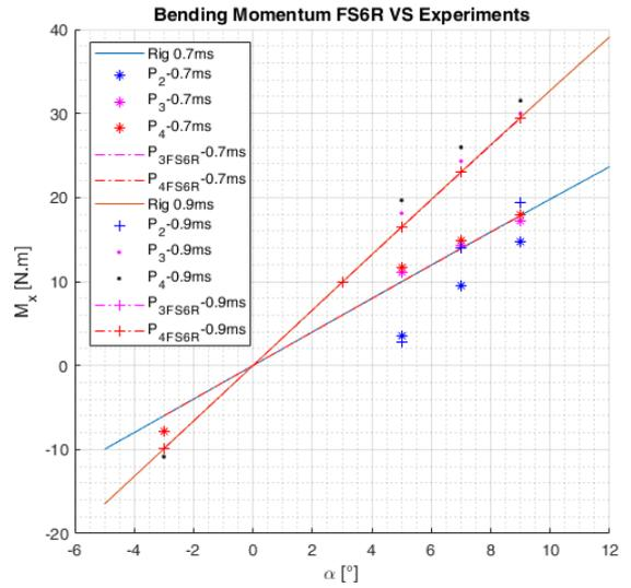
Figure 14: Experimental bending moment compared to FS6R for P<sub>2</sub>, P<sub>3</sub> and P<sub>4</sub>.
