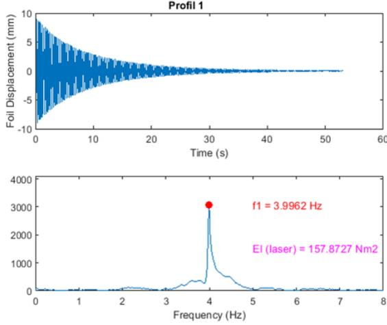
Figure 7: Vibration response of P1, test  $vib_1$ .
