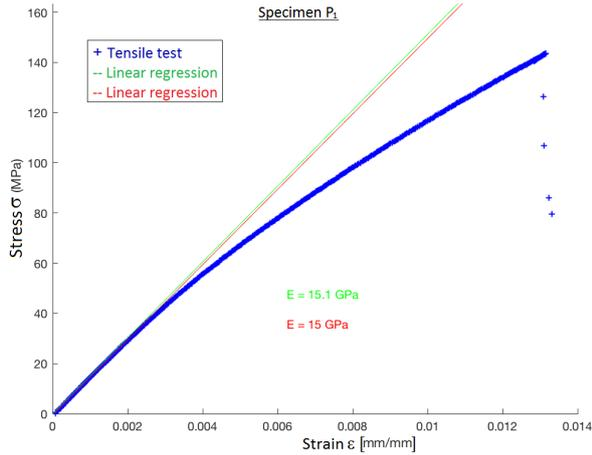
Figure 8: Stress vs strain for tensile test on the specimen layout  $P_1$ .
