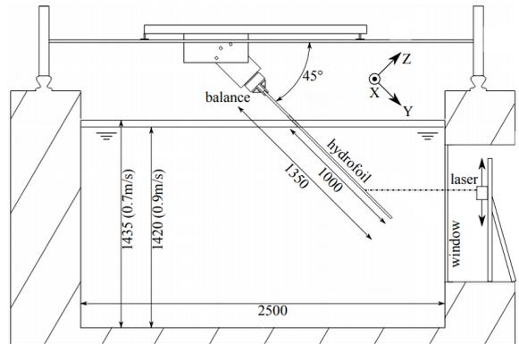
Figure 11: Hydrodynamic flume used for hydrodynamic experiments showing an hydrofoil mounted on the balance at 45° and the laser.
