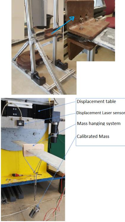
Figure 4: Bending and vibration experimental setup.
