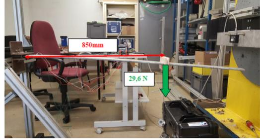
Figure 6: Bending Test  $M_2$
