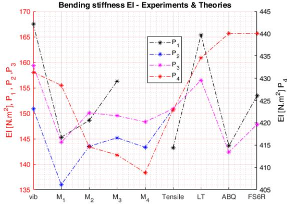
Figure 9: Comparison of Bending stiffness from numerical and experimental approaches.
