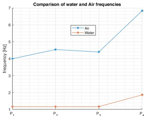
Figure 18: Hydrofoil natural frequencies in air and water.
