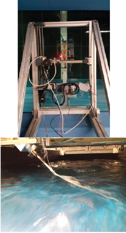
Figure 12: Hydrodynamic experiment showing the foil clamped on the balance with the strain gauges and the laser.
