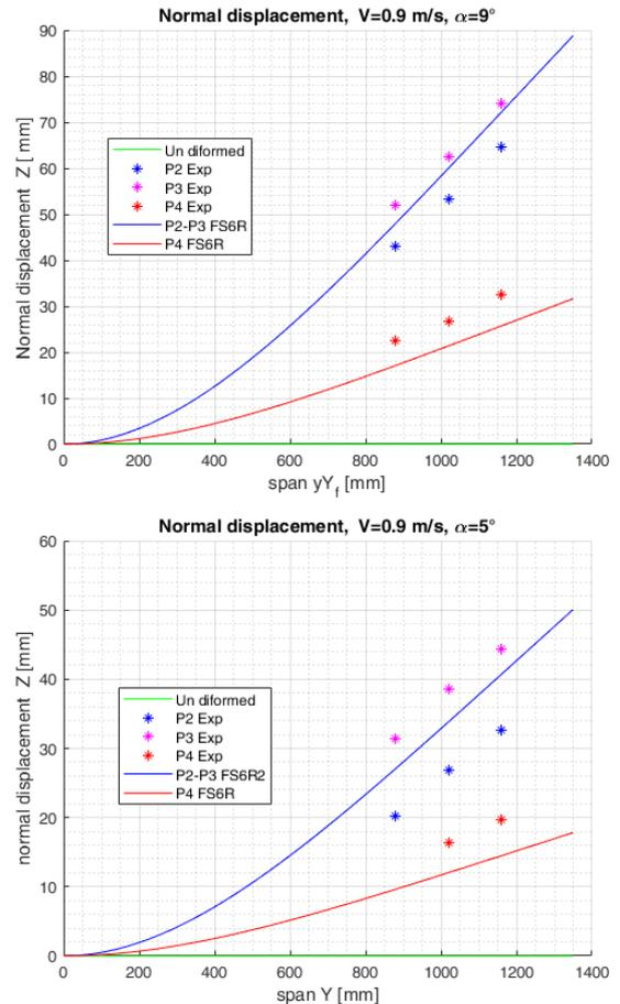
Figure 15: Displacements of the foils normal to the span, computed with FSI simulation.
