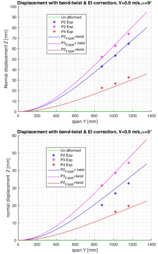
Figure 16: FS6R VS experiments: displacements for  $P_2$ ,  $P_3$  and  $P_4$  .
