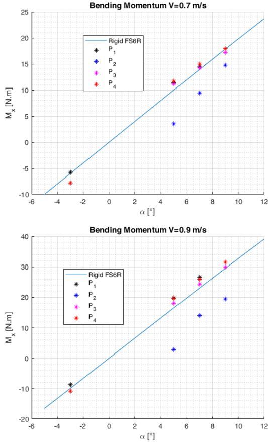
Figure 13: Experimental bending moment compared to the rigid calculation with FS6R.
