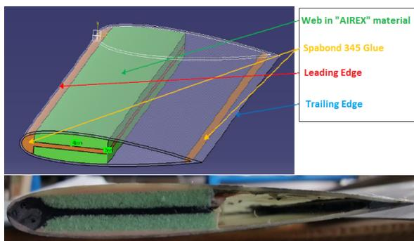
Figure 2: Hydrofoil composition and  $P_2$  manufactured section.
