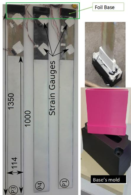
Figure 3: Finished hydrofoil with stain gauges location showing the foil base in black. Along side is the black mold and the pink 3D printed piece.
