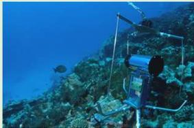
Rotating video system (STAVIRO). The system provide a 360° view divided in 6 frames of 30s (3 min per full rotation) replicated 3 times. In each frame of 30s, every species was counted within a 10m radius (5m radius for species known to be smaller than 20cm). These fish count were used to calculate taxonomic diversity indexes such as total abundance, species richness, Shannon diversity index, Simpson diversity index and Pielou equitability index.
