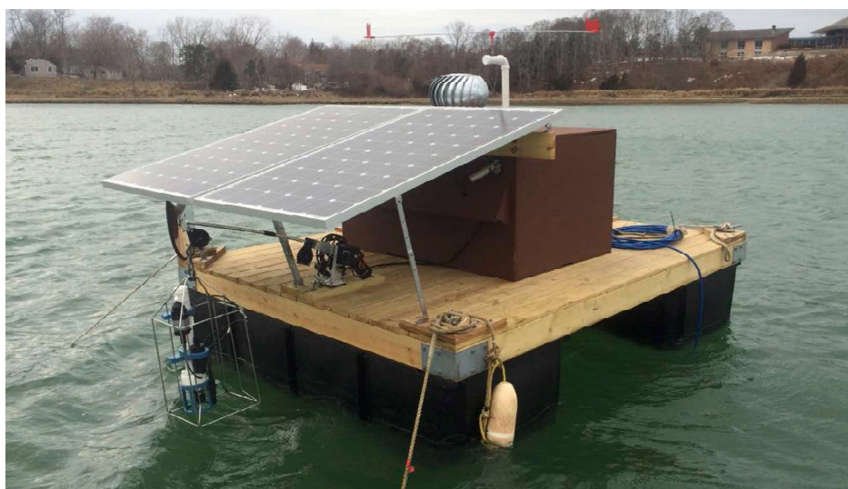
Solar powered raft platform for uncabled IFCB deployment for Alexandrium and Dinophysis studies in Salt Pond, MA (USA). The submerged IFCB (and other instruments) is raised and lowered with an automated profiling winch. (Photo: M. Brosnahan)
