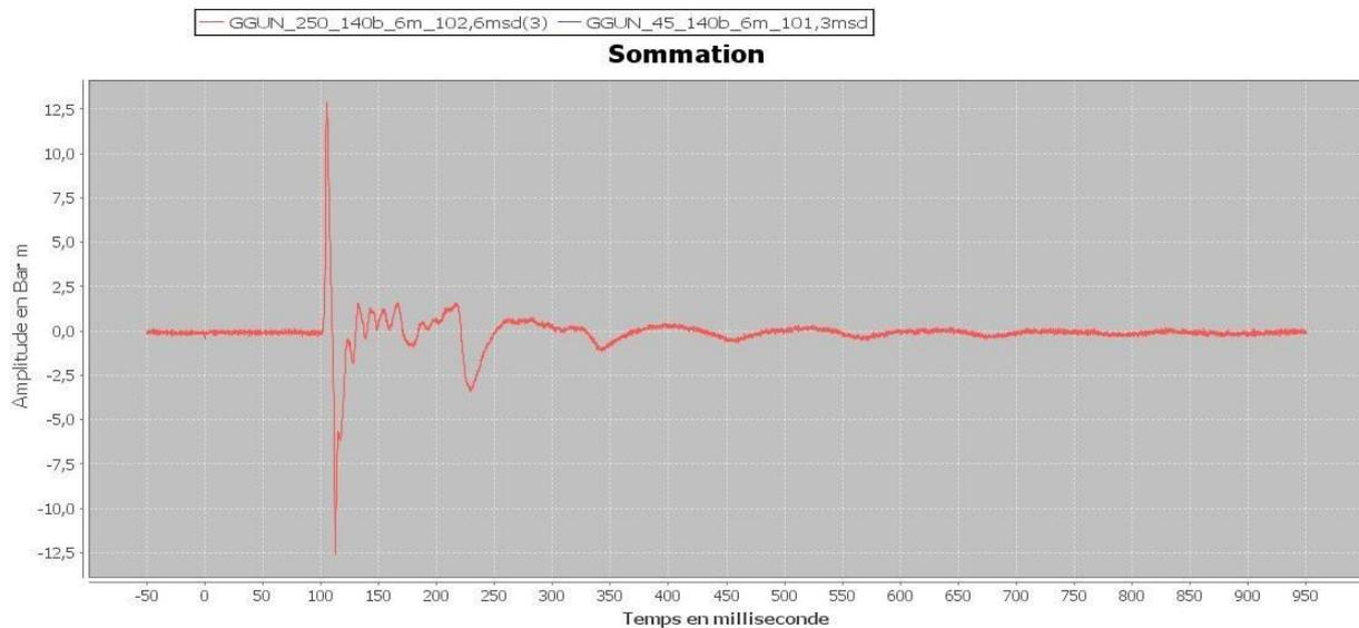
Figure 5: Acoustic signature (*Sisource* simulation) of the source made up of 4 *GGUN* air guns (3x250 in<sup>3</sup> + 1x 45 in<sup>3</sup>)
