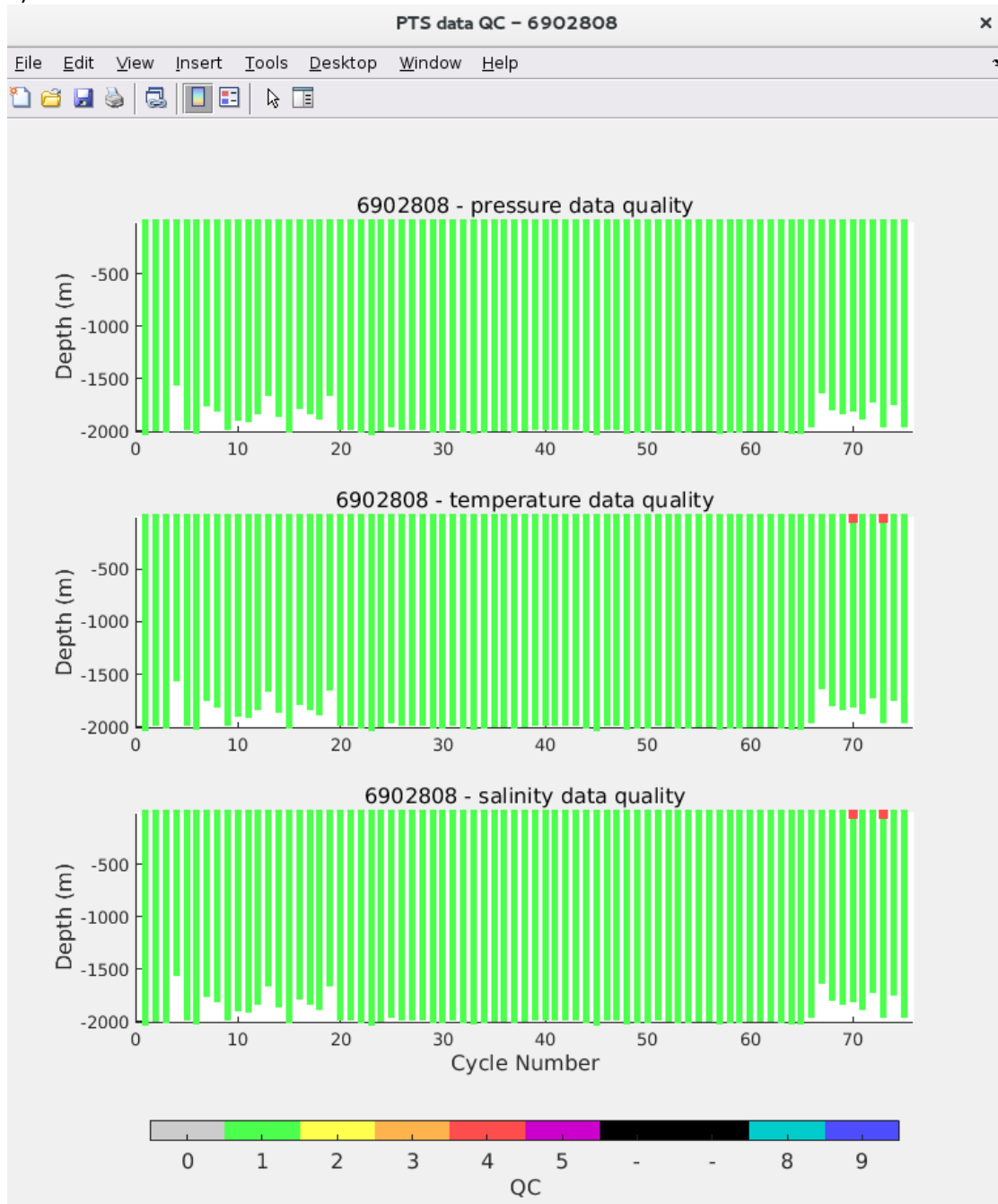
Figure 4. (saved as “DOXY_PLOT_PTS_QC...”) Time evolution as function of the float cycle number, of the vertical profiles of quality control (QC) of pressure (upper plot), temperature (central plot) and salinity (lower plot). QC range from 1 (green) to 9 (blue).
