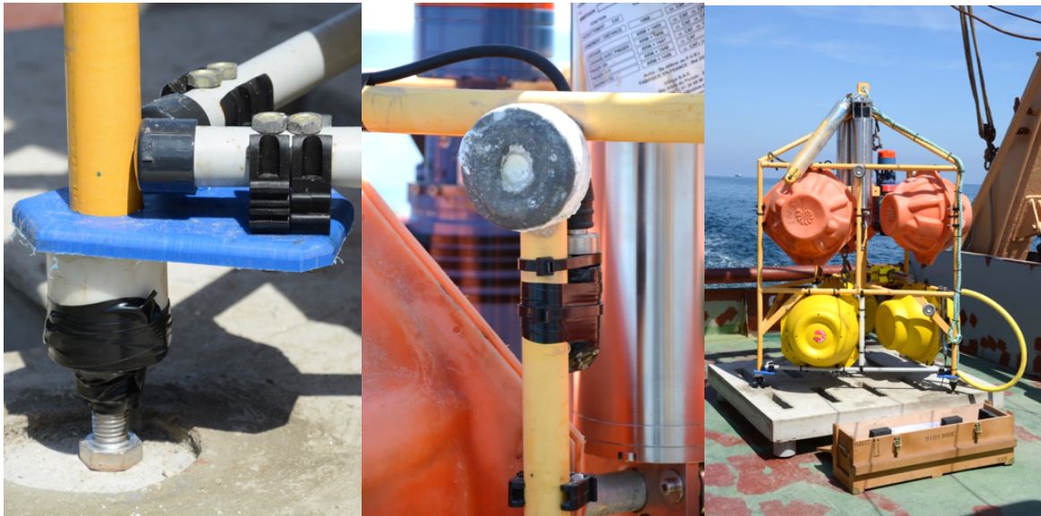
Figure 4: Instrumented frame before redeployment. (left) Refit foot; (center) Oxygen sensor; (right) Assembly ready for launch
