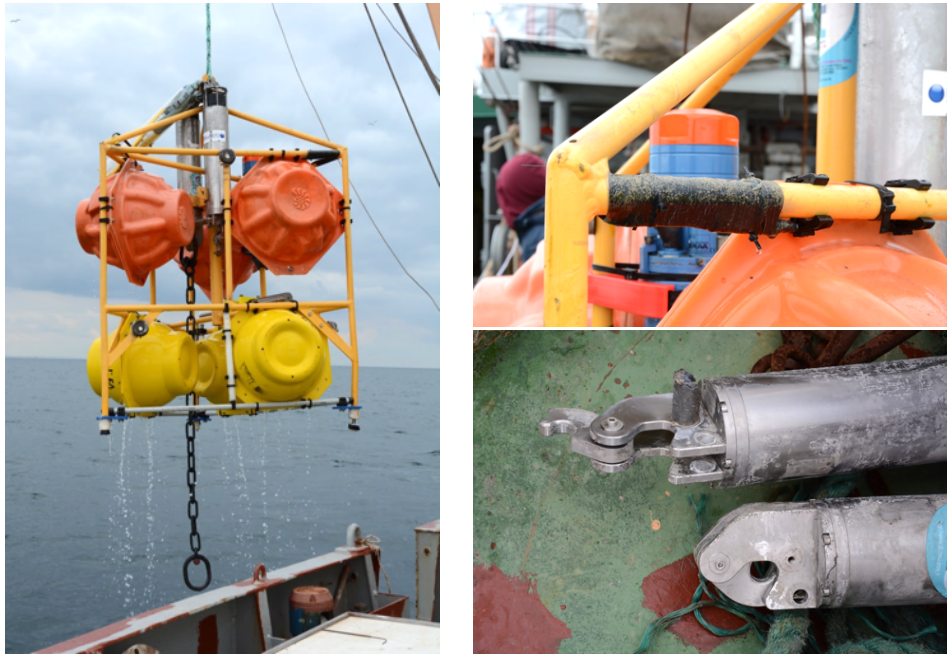
Figure 2: Recovery of instrumented frame. (left) frame is lifted on board; (top right) dust accumulation on frame; (bottom right) encrusted acoustic releaser hooks
