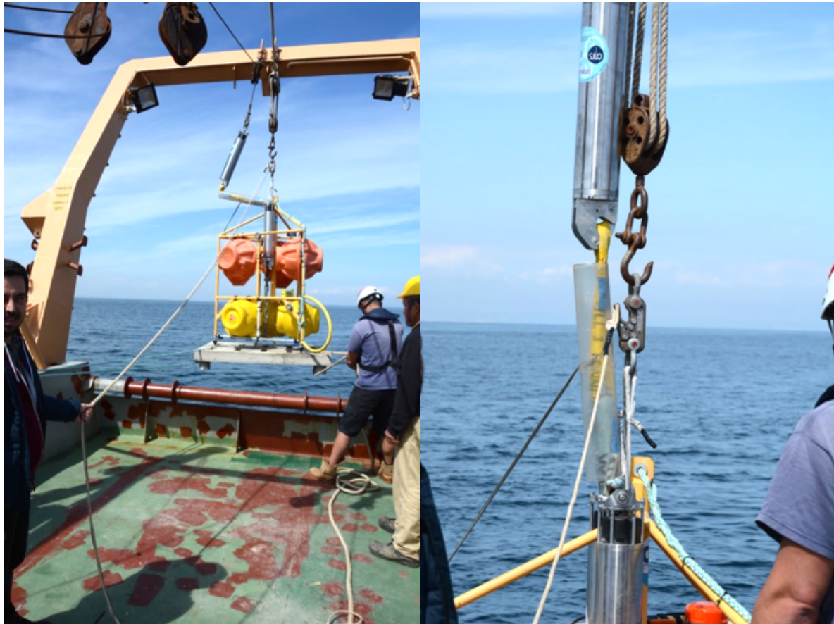
Figure 5: Deployment setup. (Left) Hoisting frame overboard on Seacatch quick-release hook; (Right) Transferring weight to the acoustic release system attached to the main cable
