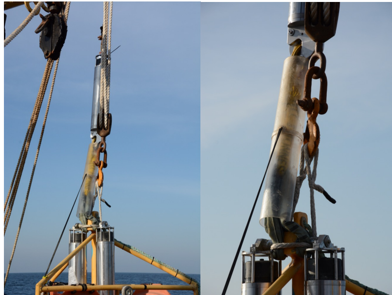
Figure 4: Deployment setup. (Left) complete view of hoisting assembly with hook and tackle used for lifting the device overboard and acoustic releaser on steel wire for used for lowering and deployment at the seafloor; (Right) detail of hook assembly
