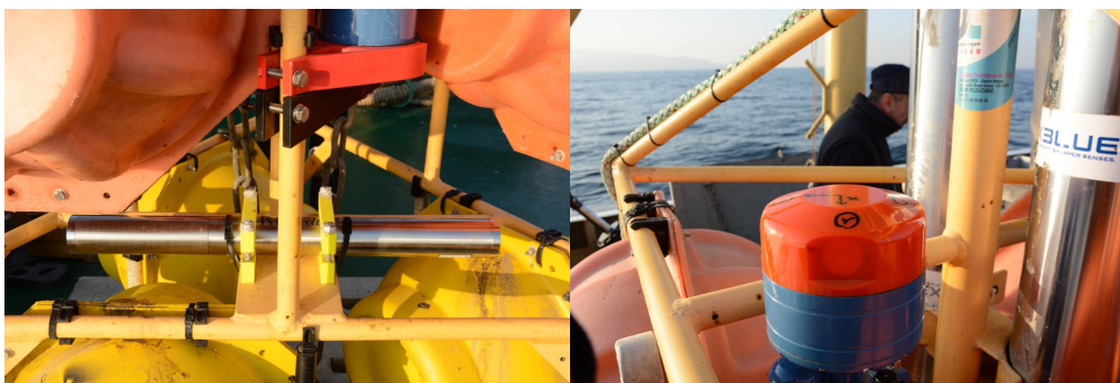
Figure 3: Instrumented frame before redeployment. (left) RBR sensor; (center) Seaguard Z-pulse sensor with XY orientation and transducer number indicated.
