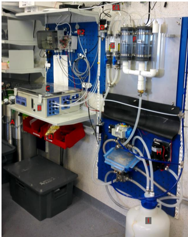
Figure 3.3.2. SuperCO 2 -system at Utö (the setup at Silja Serenade is similar, except the system for water outflow requires an additional pump, which is placed after the “exhaust water” tank). After testing several different setups, FMI has found the current pCO 2 measuring setup operating with little maintenance required. No plans to change the instrument planned. During the summer 2019, FMI plans to test the influence of inlet tube system on observed pCO 2 concentrations. As labeled: A) Reference gases, B) Instrument with LI840A gas analyzer inside, C) Tablet computer for operating the system, D) Water separator unit, E1) air filter (sample air in), E2) air filter (sample air out), F) Equilibrator chambers, G) Rotameters, H) washing pump, I) washing liquid storage bottle.
