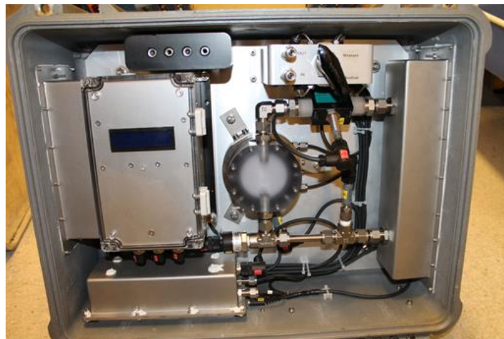
Figure 3.3.1. An example of a Franatech p\text{CO}_2 sensor system. The leftmost part contains the electronics, datalogger and display. The circular object in the middle is the equilibration chamber. And the detector lies along the bottom of the case. Water inlet and outlet on the right side of the unit with water pressure and water detector mounted. On the top the gas interface for calibration.
