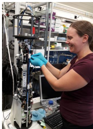
Figure 3.2.4. Replacing pumps, tubing and renewing reagent bags for biocide and calibration beads are occasional tasks for Imaging FlowCytobot user.
