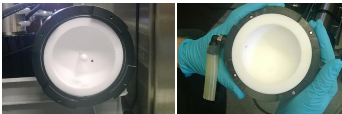
Figure. 3.2.3. The measurement cavity of absorption meter OSCAR is covered with reflective material (TFE). It need to be frequently cleaned with NaOCl, pure ethanol and lint-free tissue.
