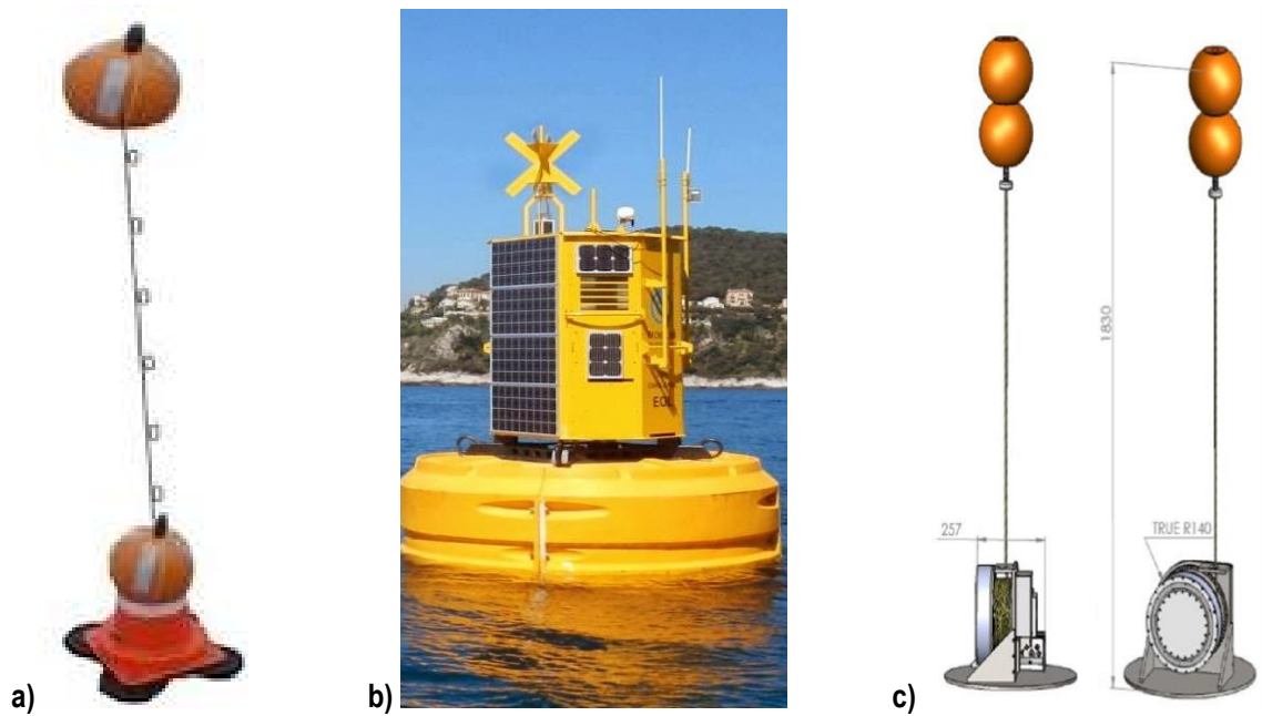
Figure 3.4.1. Example of coastal profilers: (a) Mastodon 2D, (b) EOL buoy, (c) YOYO
