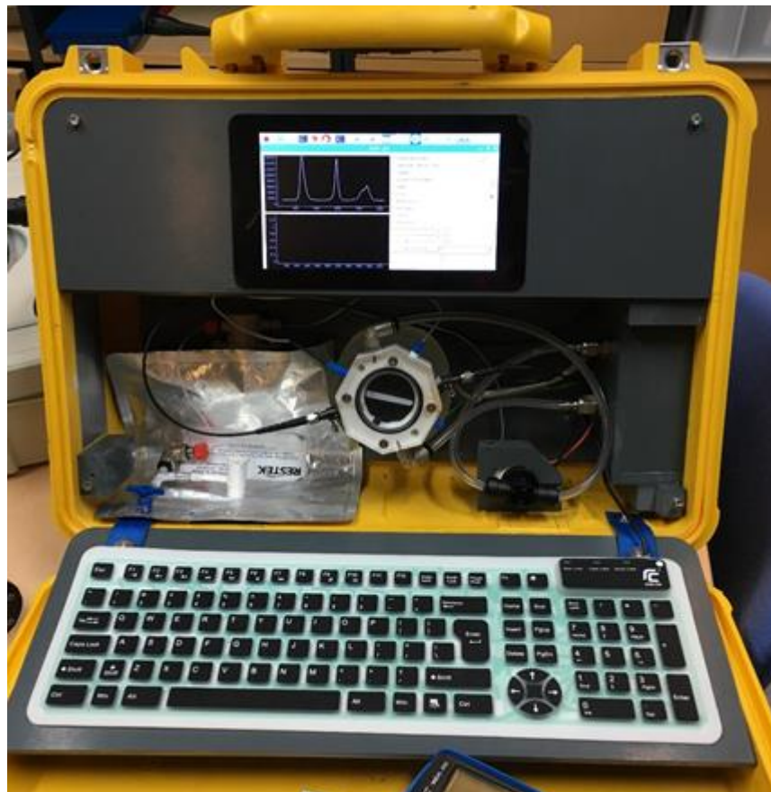
Figure 3.3.4. NIVA spectrophotometric pH system. The system includes (from top left to bottom right: touch screen display of Python GUI, gas impermeable foil reagent bag for indicator dye, cuvette with stir bar, and pump for indicator dye. Not shown but present in the top compartment: Raspberry Pi, spectrophotometer.
