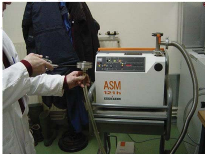
Figure 5. Helium leak detection equipment
