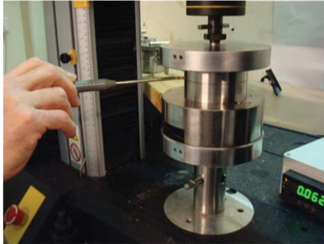
Figure 6. Helium detection during compression loading of joint in test fixture.
