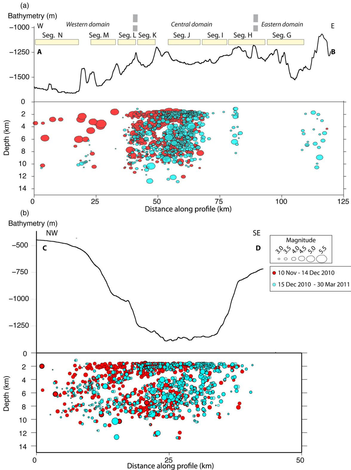
**Figure 4.** Hypocentre and bathymetry cross-sections, locations indicated in Fig. 3(a). (a) EW-trending cross-section along the ridge (b) NW-SE-trending cross-section along the segment J axis. The horizontal scale is not the same for the two profiles. The arrows on the profile (b) indicate the area of low superficial activity.
