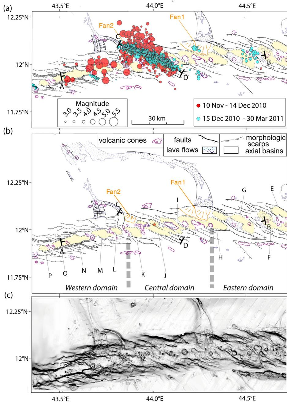
**Figure 3.** (a) Seismicity recorded from 2010 November 10 to 2011 March 30. (b) Morphotectonic features from Audin (1999); location in Fig. 1. The orange star indicates the location of the melted optical wire and hot surface sea water observations (see Section 6). (c) Shaded bathymetric data of the area under study.
