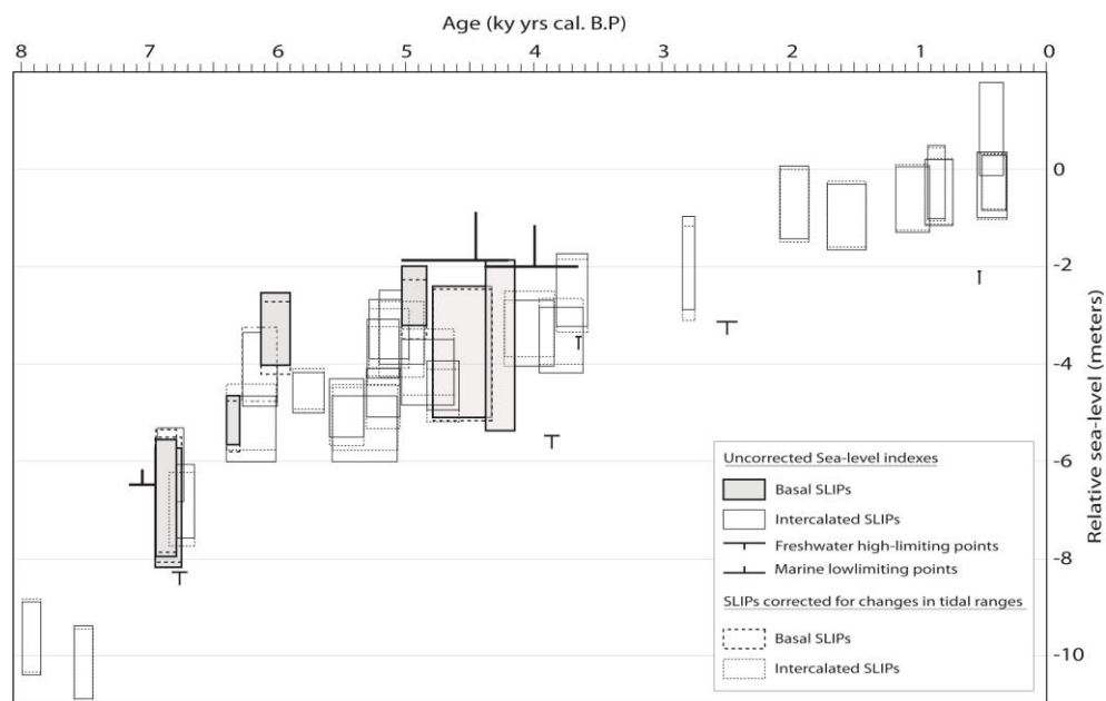
Figure 14 - Sea-level index points uncorrected (plain boxes) and corrected (dotted boxes) for paleo tidal range changes through the last 8 ky cal. B.P.
