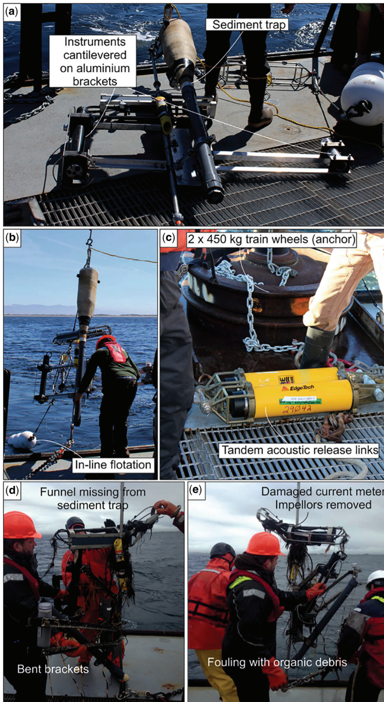
Fig. 3. Photographs of a sediment trap and inline instruments placed within turbidity currents from Monterey Canyon. (a) Pre-deployment photograph of a sediment trap and instruments fitted on cantilevered aluminium brackets. (b) Deployment of a sediment trap. (c) Detail on anchor weight (train wheels) and acoustic release links, which were placed 3 m above seafloor. (d, e) Sediment trap and instrument brackets following retrieval, showing damage and fouling during interaction with turbidity currents.
