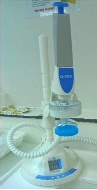
A photograph of a Q-POD ultra-pure water dispenser. It is a white, floor-standing unit with a blue top section. It has a digital display and a control panel on the front. A white coiled tube is connected to the side.                                                                     |
