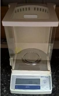
A photograph of a precision analytical balance. It has a white top with a transparent protective cover and a digital display on the front. The weighing pan is visible inside the cover.                                                                                                      |
