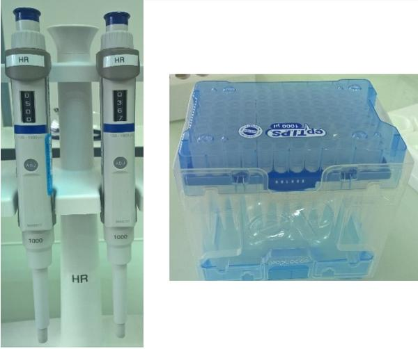
Two photographs showing Eppendorf Research plus pipettes. The left image shows two pipettes, one labeled 'HR' and '1000', standing on a white stand. The right image shows a clear plastic box containing a large quantity of blue pipette tips, with the Eppendorf logo visible on the lid. |
