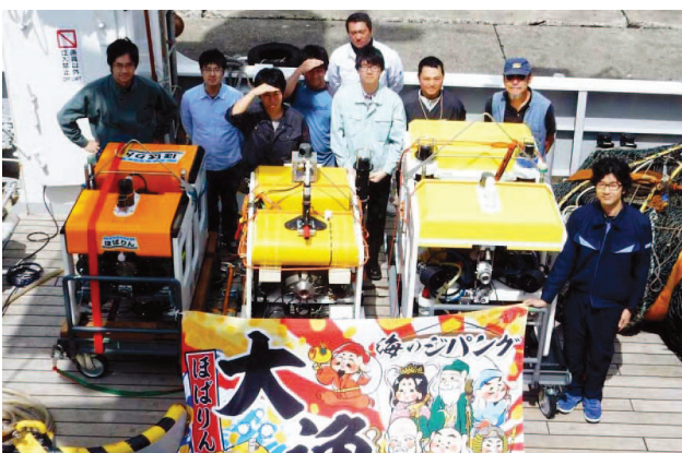
Fig. 15. Three Tuna-Sand class AUVs, Tuna-Sand, Hobalin ( L = 1.2 m, W = 270 kg), and Tuna-Sand 2 ( L = 1.4 m, W = 380 kg), surveyed benthos in the Sea of Okhotsk.
