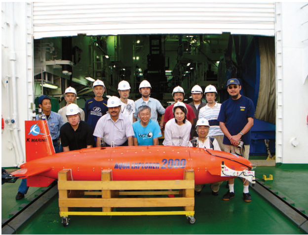
Fig. 4. Aqua-Explorer 2000 ( L = 3.0 m, W = 300 kg) on the deck of the R/V Kairei.
