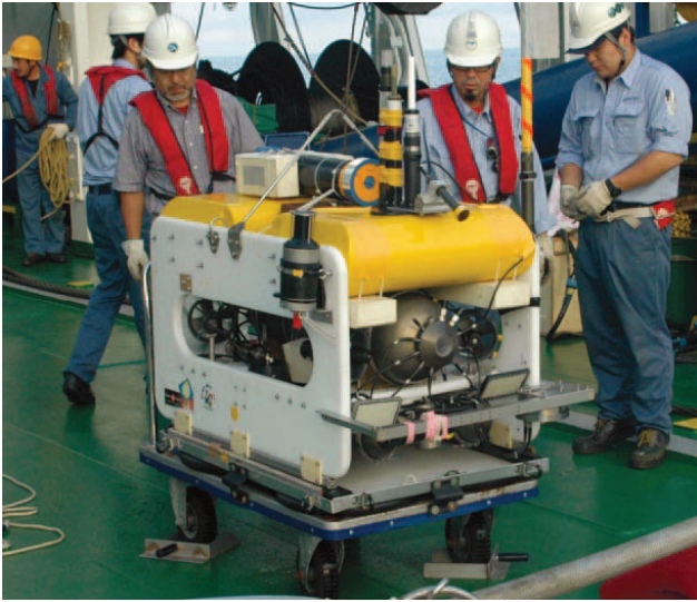
Fig. 10. Tuna-Sand ( L = 1.1 m, W = 240 kg) is the first Tuna-Sand class vehicle constructed in 2007.
