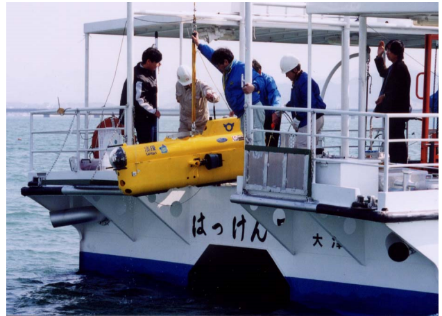
Fig. 9. Tantan ( L = 2.16 m, W = 180 kg) surveyed Lake Biwa, the largest lake in Japan.
