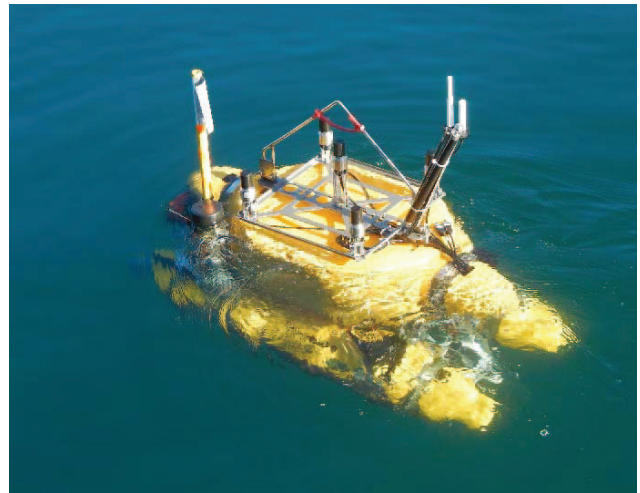
Fig. 16. Hovering AUV Tri-TON 2 ( L = 1.4 m, W = 300 kg).
