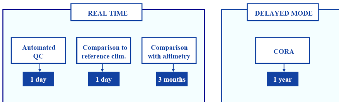
Figure 4: Quality control procedures during the real time and delayed mode validation chain.
