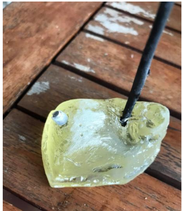
Abrasion tests of the LoRa antenna and resistance of the electrodes and resin to strong shocks
