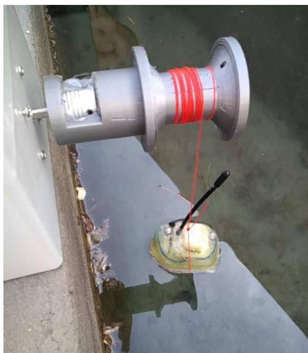
Tag in surface position on the test bench deployed in Kelsonia © IFREMER
