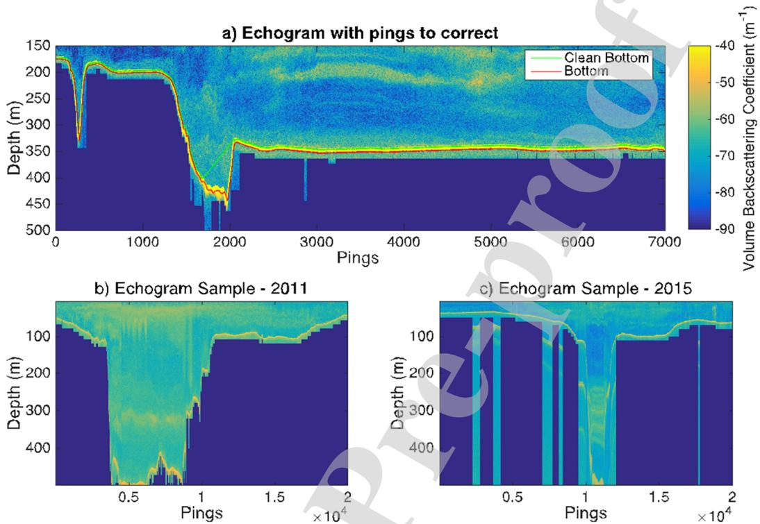
**Fig 2.** (Color online) Echogram extracted from the acoustic sea survey used in the study. (a) An example in which the automatic procedure for bottom detection (green line) has failed around ping 2000. (b) Random samples from the 2011 and (c) 2015 echograms, with the same ping size and cell number; showing differences with respect to the settings for NaNs (“not a number”, strong blue color) below the bottom. Unit: see color bar in panel (a).
