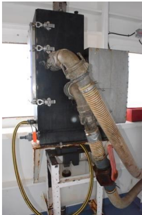
Figure 31 : The Continuous Underway Fish Eggs Sampler.
