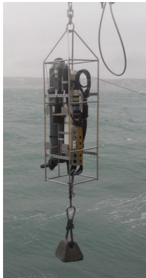
Figure 29 : Hydrological station. The SBE 19 sensor and the Niskin Bottle
