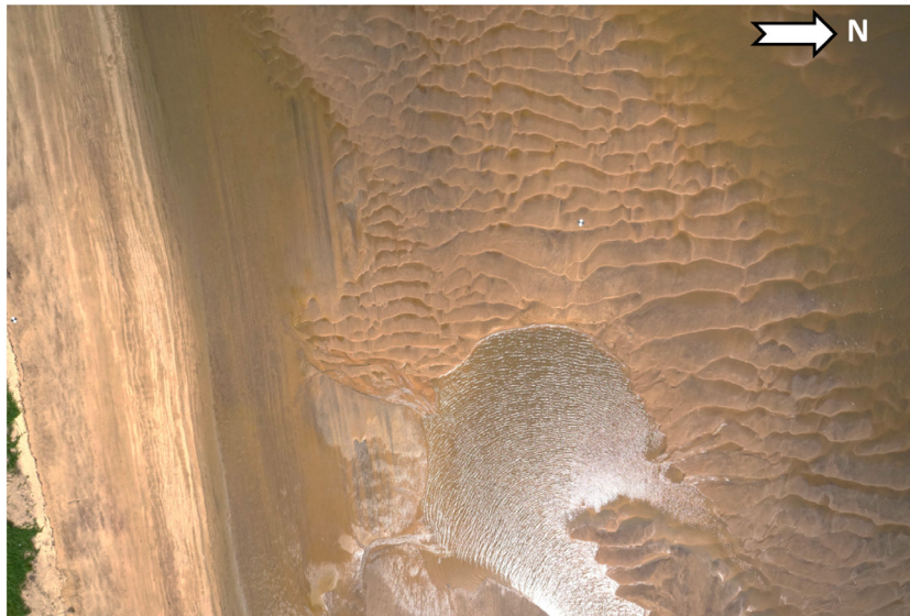
Fig. 4. Photo of 2D to 3D dunes exposed at low tide on the inner shoreface adjacent to the beach at Yalimapo (see 1 in Fig. 3). These dunes migrate eastward under the influence of ebb-dominant residual flow.
